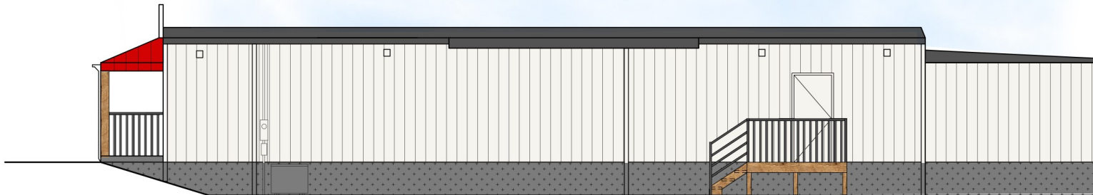
RIGHT EXTERIOR ELEVATION SCALE: 1/4"=1'-0"
